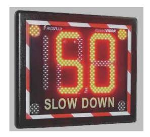
MINIVISOR 230 has been developed to display and store the speed of passing vehicles. It combines a radar sensor with a 2½ digit 7 segment LED display, the control electronics and the electricity power supply.
